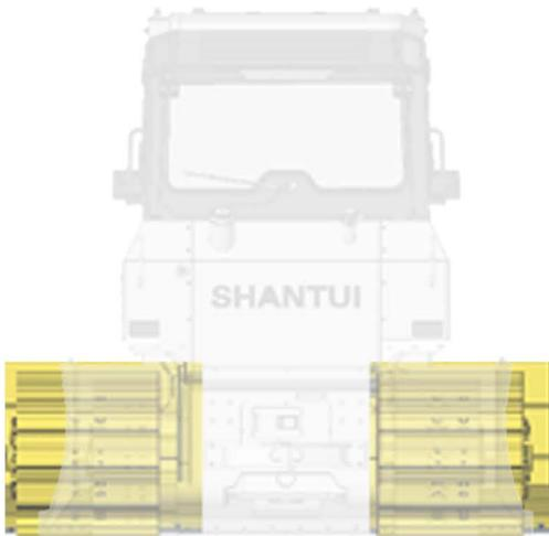
**WIDER TRACKS AND BLADES HELP DISTRIBUTE THE WEIGHT AND PREVENT THEM FROM SINKING INTO THE GROUND AND GETTING STUCK WHILE OPERATING.**
